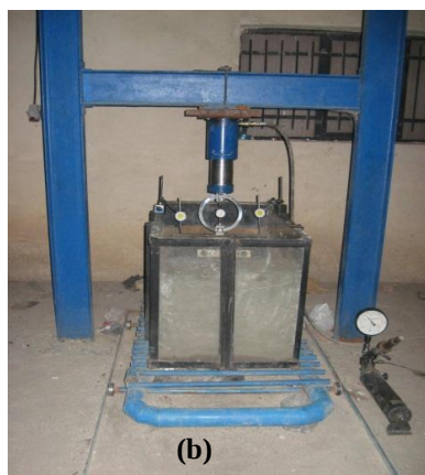
Figure 5. Vibratory tamper and test box during loading (a) Vibratory tamper (b) Loading frame and test box
