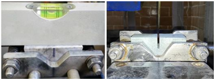
Figure 5. Notching the rock specimens
