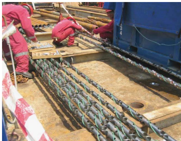
Figure 1. Loading shaped charges into perforating guns [6]
