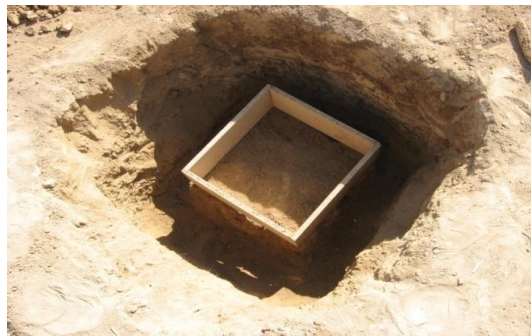
Figure3. Monolithic sampling method
