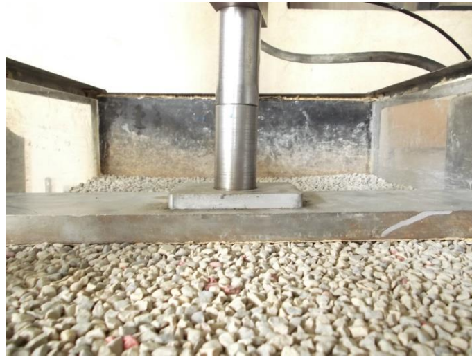
Fig. 4. Assembly of the shaft and the base plate installed on the footing
