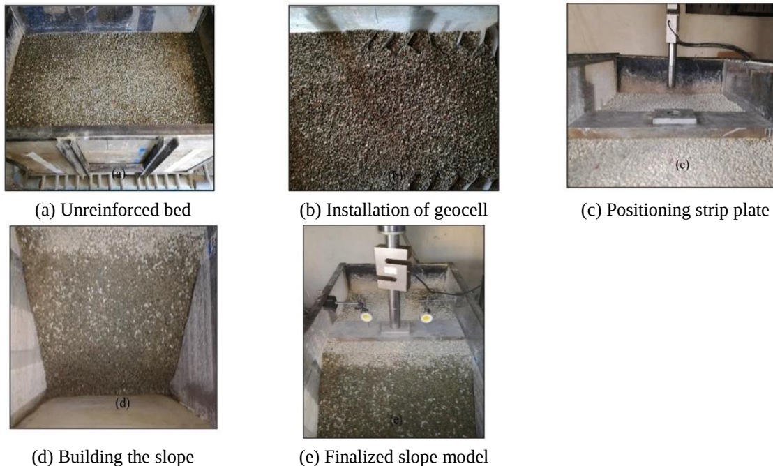
Fig. 5. Test bed preparation sequence
