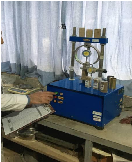
Fig. 7. Device of unconfined uniaxial compressive strength test in the present study
