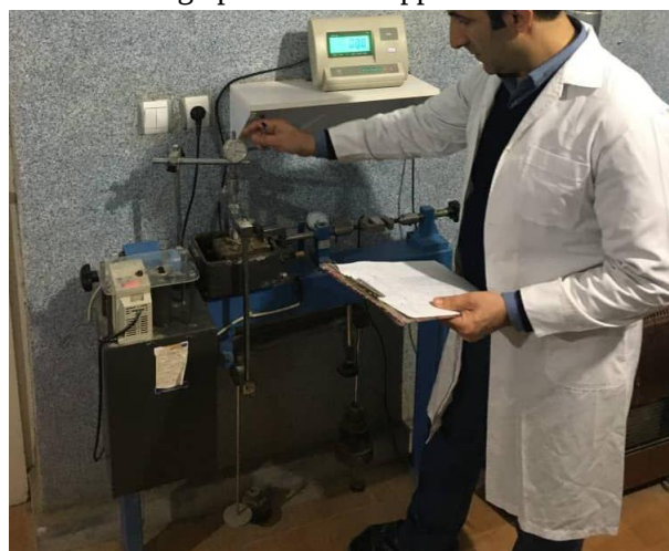
Fig. 8. Device of direct shear test used in the present study
