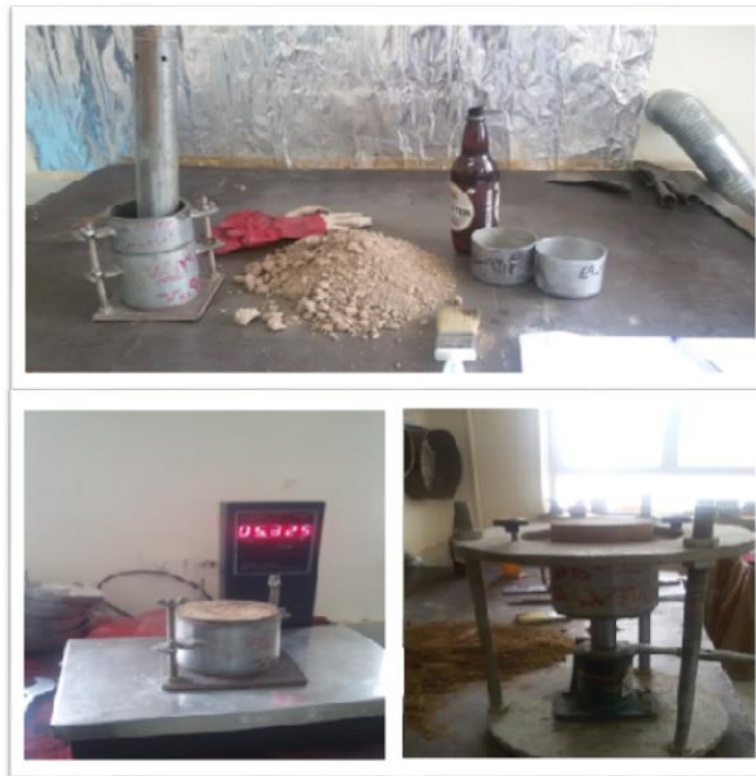
Fig. 6. Compaction tests device used in the present study
