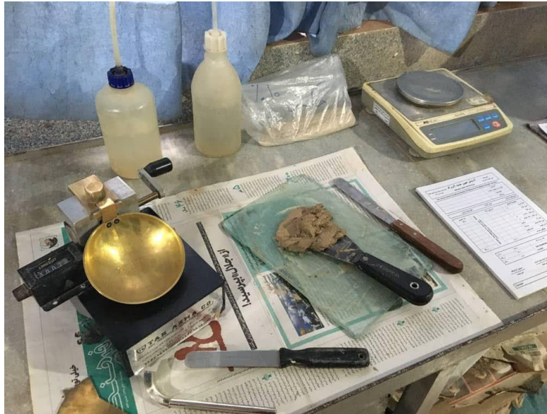
Fig. 5. Device and procedure of Atterberg tests
