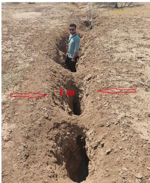
Fig. 4. Longitudinal and deep cracks in the Eshtehard plain (Fathabad region)
