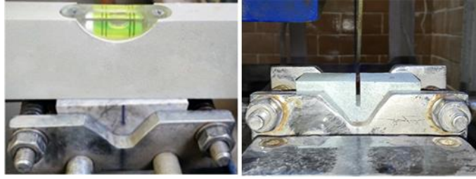
Figure 5. Notching the rock specimens
