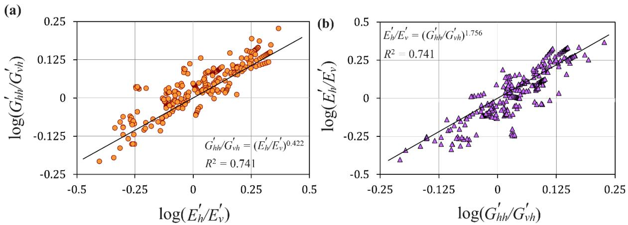
Fig. 2. The reciprocal plotting the anisotropy ratios (a)  $G'_{hh}/G'_{vh}$  versus  $E'_h/E'_v$ , and (b)  $E'_h/E'_v$  versus  $G'_{hh}/G'_{vh}$  in log scale by performing linear regression analyses for evaluating their correlations
