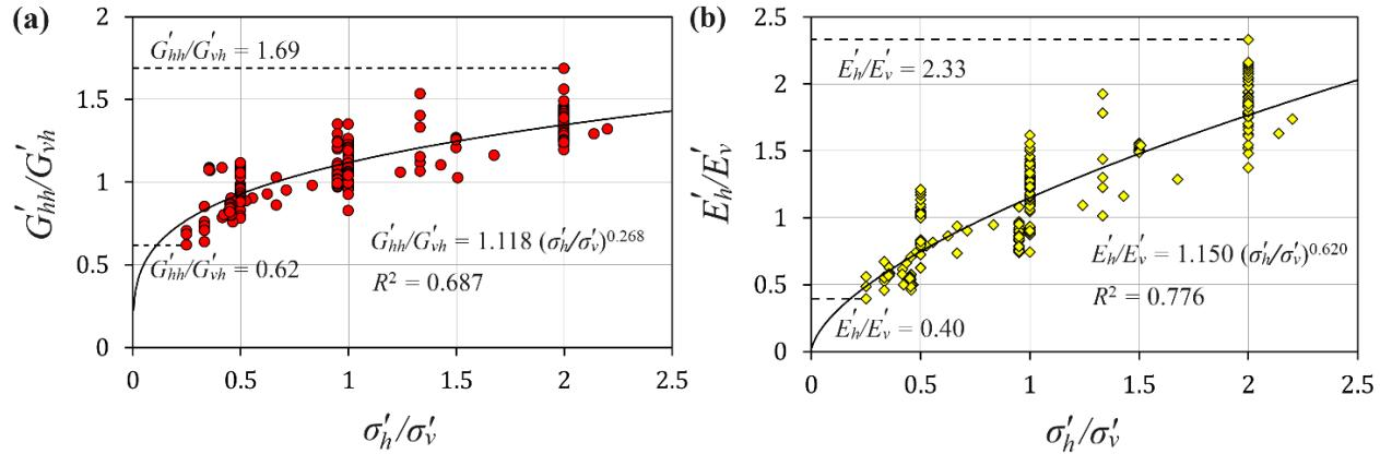
Fig. 1. The variations model of (a) shear modulus anisotropy ratio  $G'_{hh}/G'_{vh}$ , and (b) Young's modulus anisotropy ratio  $E'_h/E'_v$  versus the stress ratio  $\sigma'_h/\sigma'_v$  in cohesionless soils
