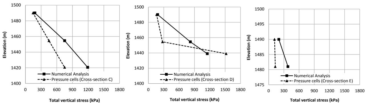
**Fig. 13.** Variation in the total vertical stresses obtained from the numerical analysis and the pressure cells along the height of the dam at the end of construction for cross-sections a) C, b) D and c) E
