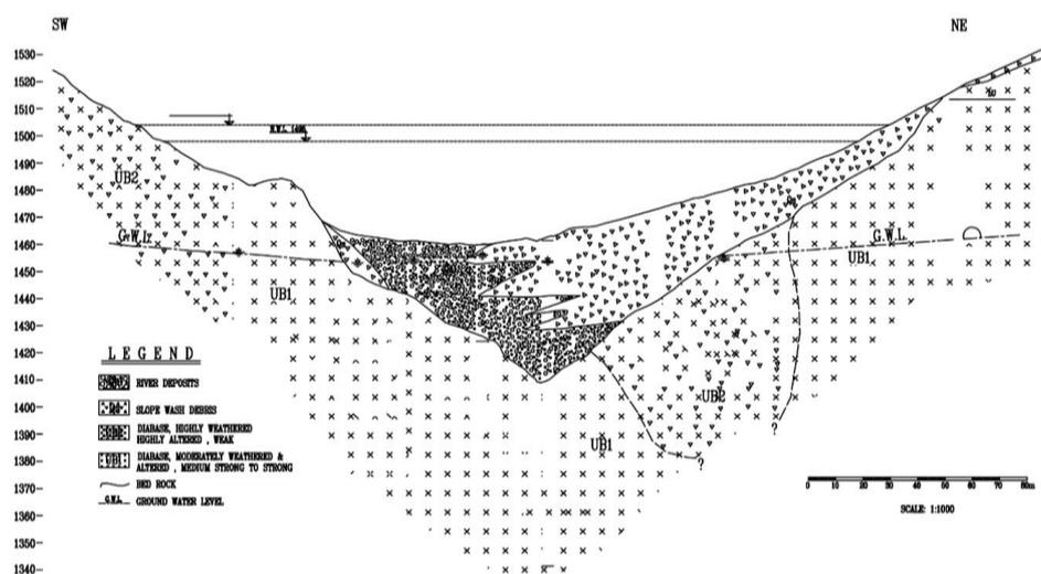
**Fig. 1.** Engineering geology profile of the dam site
