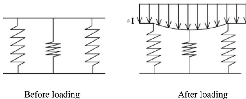
**Fig. 11.** Simulation of soil stiffness around the instruments
