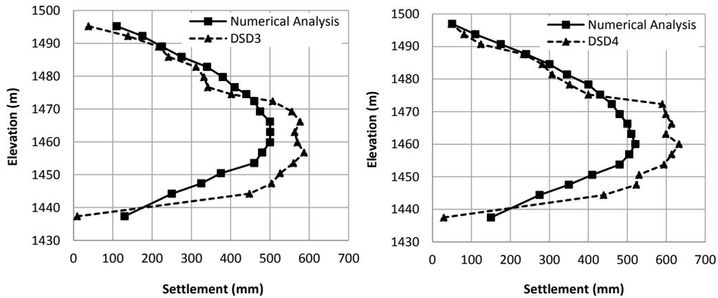
**Fig. 9.** Comparison of the settlements recorded by the instruments and the numerical analysis results for cross-section D
