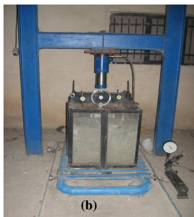
Figure 5. Vibratory tamper and test box during loading
