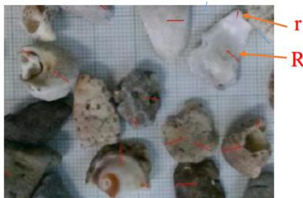
Figure 7: Measuring the radius of the sharpest corner of angular aggregate and the radius of circle inscribed in the aggregate using JMicrovision software.
