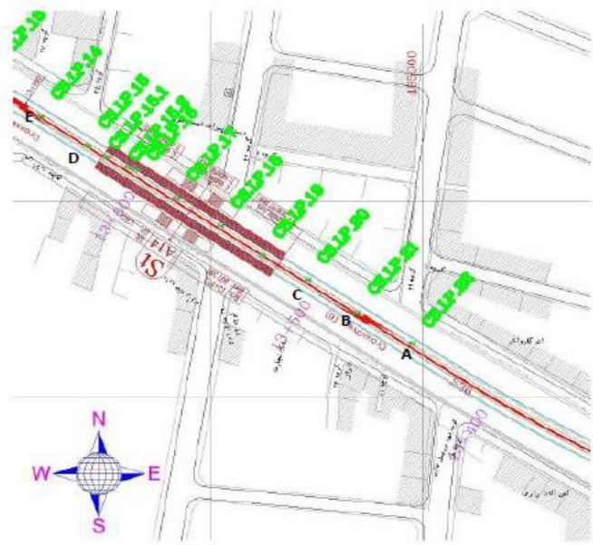
Figure 15. The installation location of settlement gauges at the studied sections [15].
