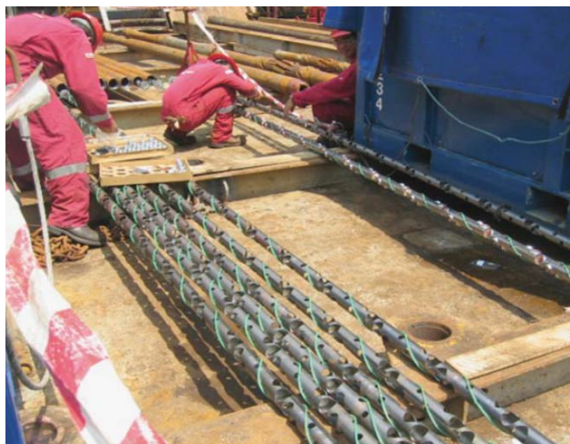
Figure 1. Loading shaped charges into perforating guns [6]
