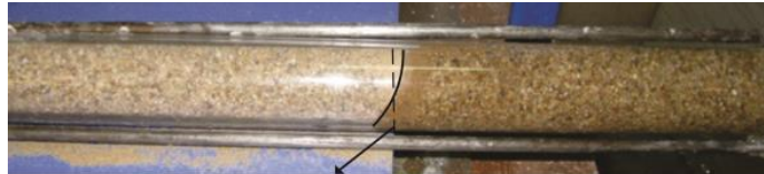
Figure 1. The reading point of the penetration length in the sample
