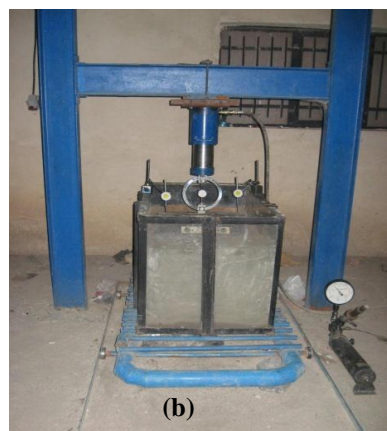
Figure 5. Vibratory tamper and test box during loading
